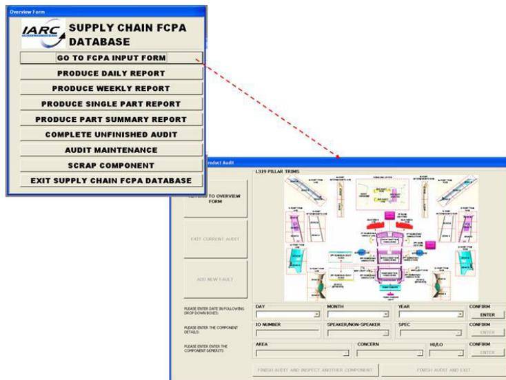
Figure 4: Audit Database Graphical User Interface (GUI)
