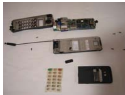
Figure 5: Product dissection example (cellular phone, OKI, 1998)
