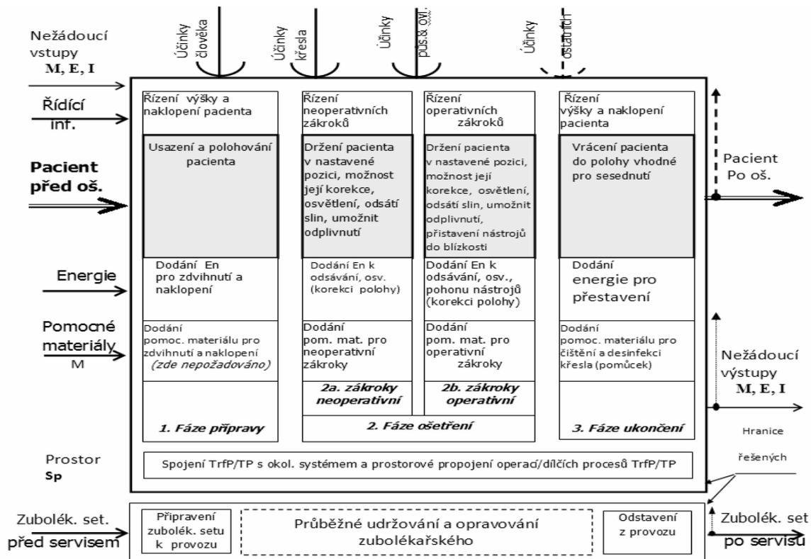
Figure 7. Operation Process for the designed technical product - Example: Dental Chair
