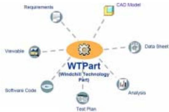
Fig.5. WTPart technology by PTC (Parametric Technology Corp.) a container for all documents concerning product numbers through its life cycle [PLM system by PTC, product information]
