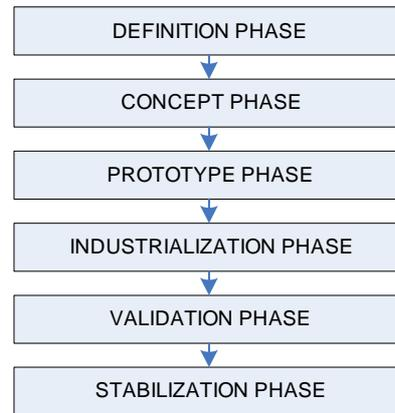
Fig.2. Example of prescriptive design model in automotive industry
