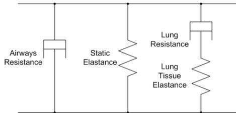
Figure 2 A mechanical diagram, modelling the pulmonary system of dogs
