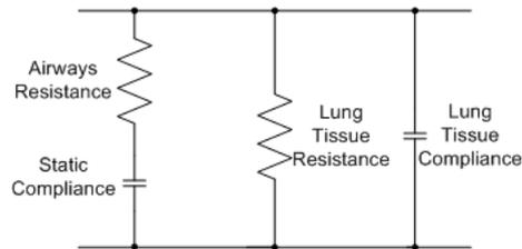
Figure 1 An electrical diagram, modelling the pulmonary system of dogs
