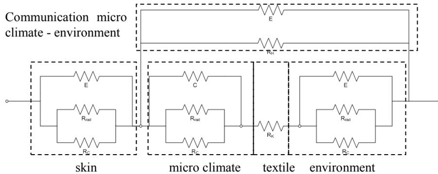
Figure 4 The heat transfer from a body through an artificial microclimate and textile to the environment
