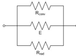
Figure 3 The heat transfer from a body to the atmosphere, using convection, radiation and sweating
