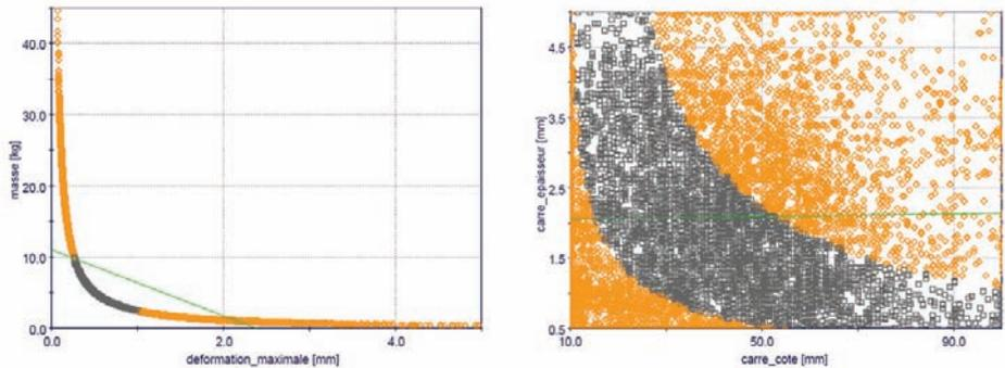
Figure 6 Results obtained with genetic algorithms for the multi-objective optimization problem. Orange color is used for solutions with excessive mass value (over than 10 kg) or excessive displacement value (over than 1 mm).
