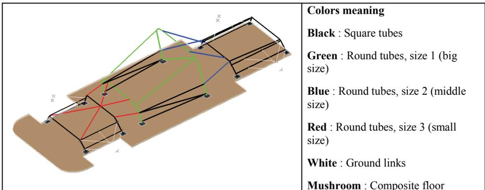
Figure 8 chassis frame design characteristics
