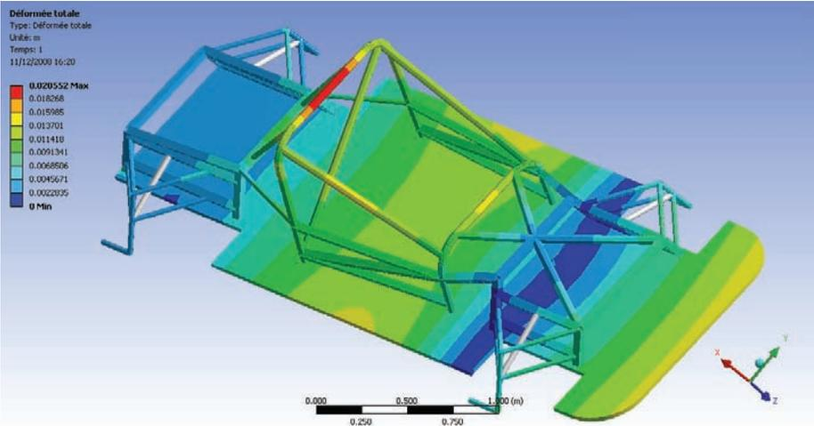
Figure 9 : F.E. calculation on the initial chassis frame
