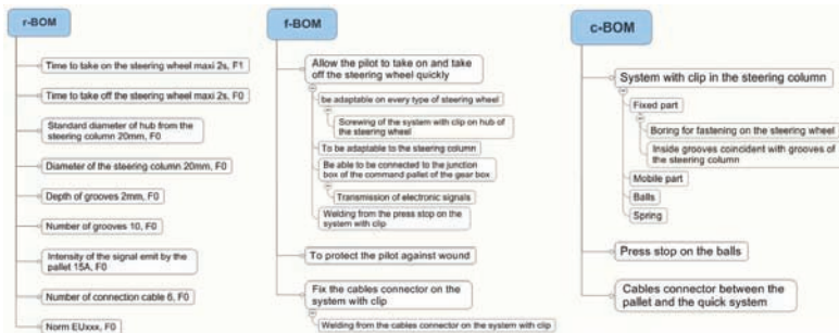
Figure 7: r-BOM, f-BOM and c-BOM of the quick system
