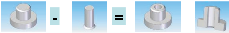
Figure 12. Vacuum = material (+) – material (-)
