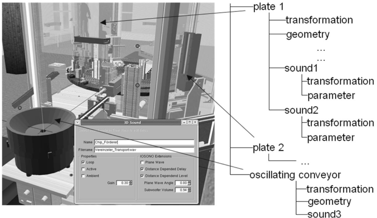
**Figure 3. Audio-visual model of a revolving automatic assembly machine**
