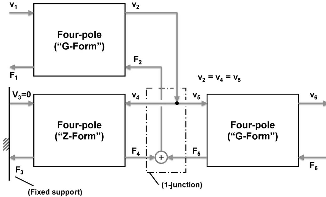
Figure 7. Coupling of four poles
