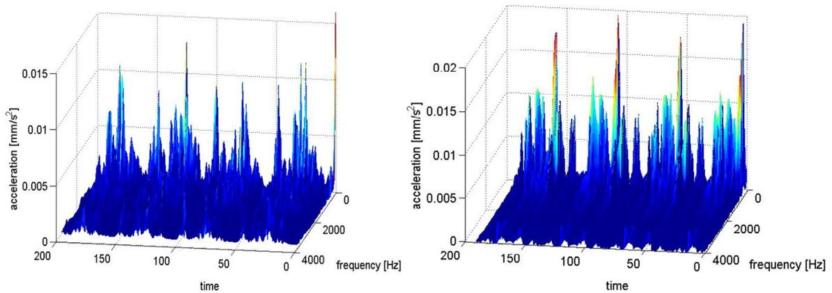
**Figure 10. Measured and simulated acceleration on the surface (side wall) of the pick-place unit**
