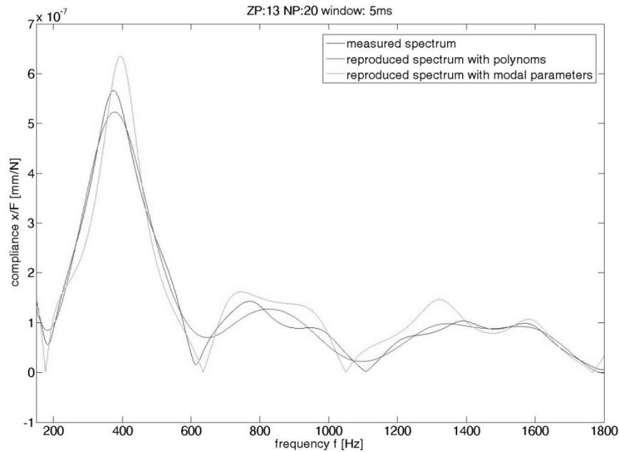
**Figure 8. Measured and reproduced transfer function**
