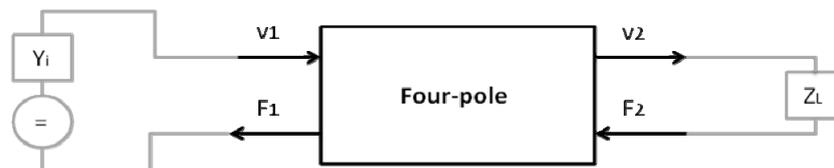
**Figure 6. Simple four pole with a source and a load impedance**
