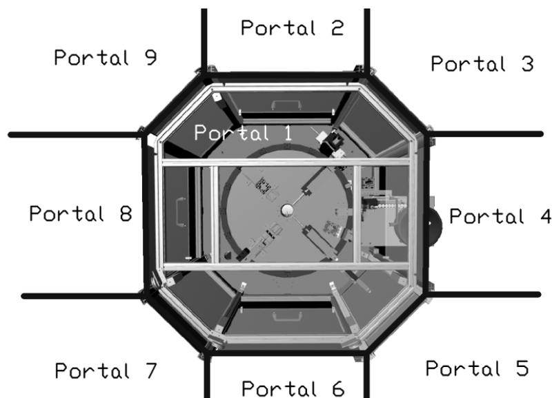
**Figure 4. Portals in the model of a revolving automatic assembly machine**
