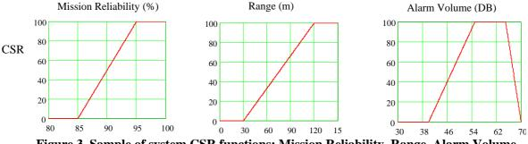
Figure 3. Sample of system CSR functions: Mission Reliability, Range, Alarm Volume
