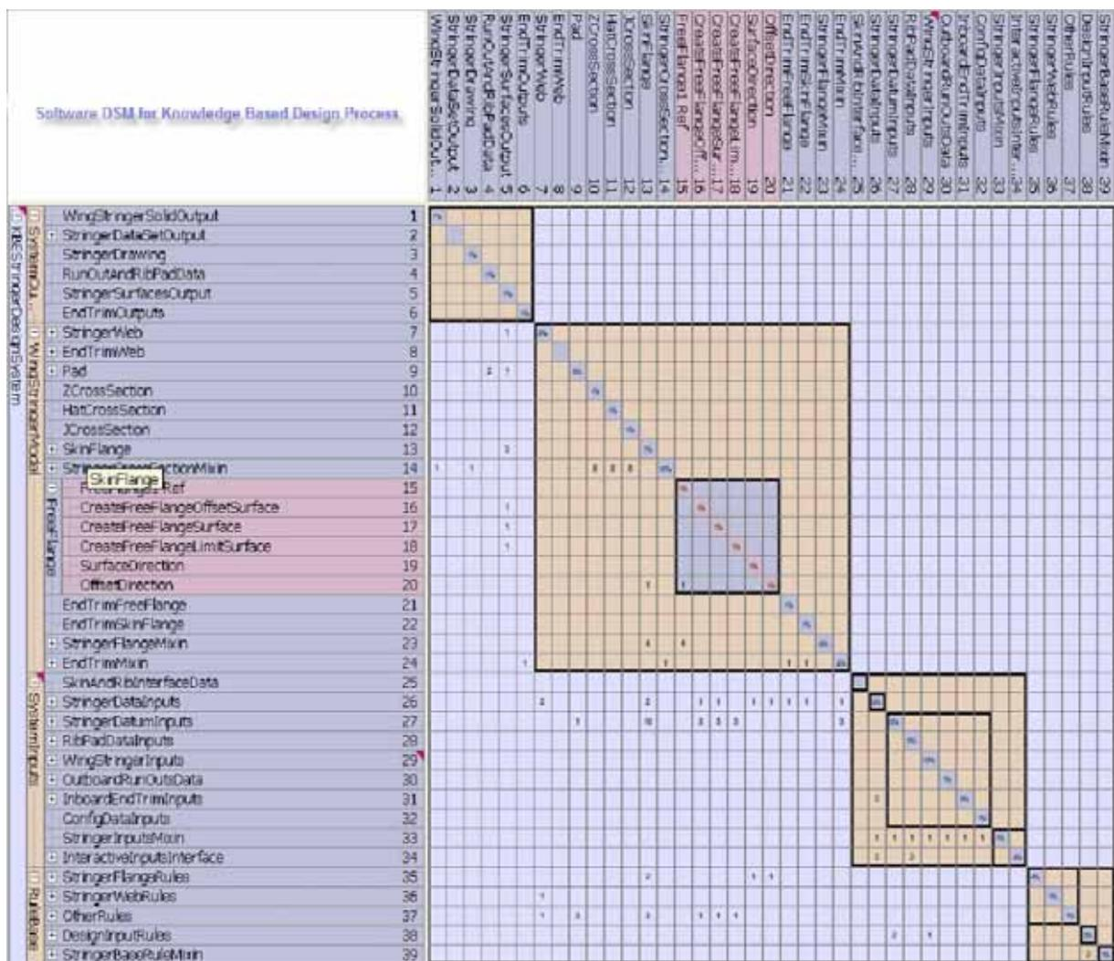
Figure 3. Corresponding software DSM for the engineering DSM in Figure 2
