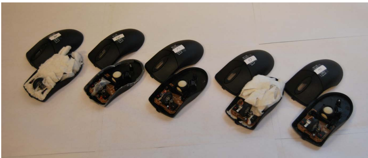
Figure 5. The sound designs of five similar products were modified. A: filled with material reducing the product's volume. B: tightening the overall assembly using tape in all joints. C: replaced the micro switch. D: replaced the micro switch, dampener below the PCB-board and reduced the product's volume. E: no modifications.
