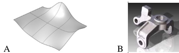
Figure 3. A digital 3D surface representation. B. A digital 3D solid model representation.
