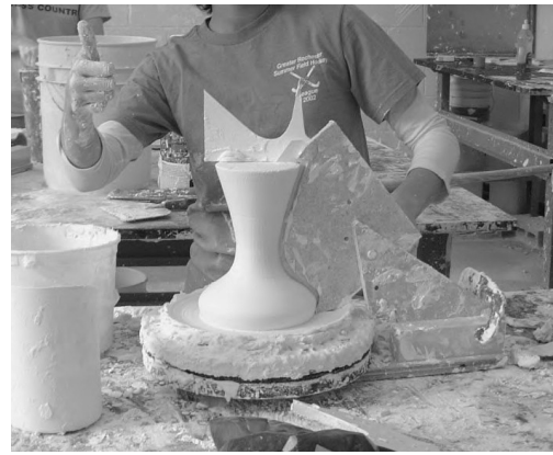
Figure 6. Turned plaster form and set-up
