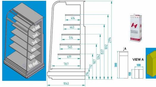
**Figure 2.** 3D Models of a vertical unit for fresh products and of a milk package.
