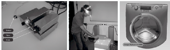
Figure 8. Mixed Prototyping application for the usability test of virtual washing machines by means of programmable interactive devices: knob, button, and slider.
