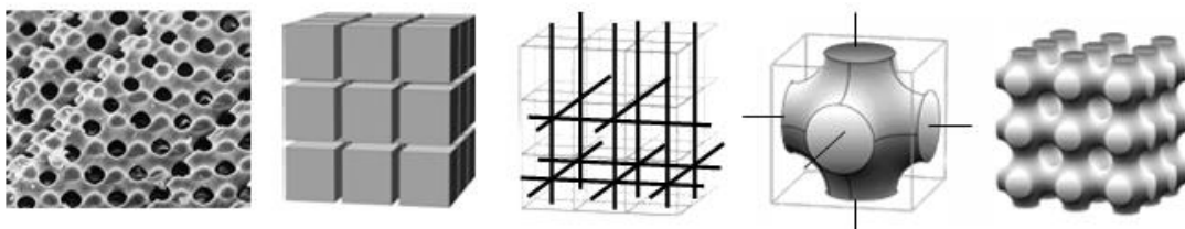
Figure 4. Basic stages of form development (from left to right). Stage 1 – Complex pattern identification (source: http://www1.chem.leeds.ac.uk/FCM/mech%20props.html ). Stage 2 – Infinite polyhedra serves as assembly logic Stage 3 – Infinite polyhedra net used as a cage for the constructive skeletal graph of the future basic unit. Stage 4 – Basic unit design inside the “cage.” Stage 5 – Inherent joint development, followed by an assembly.
