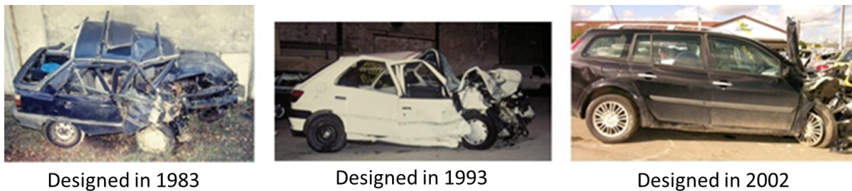
Figure 1. Evolution of car's in-depth accident analysis (65km/h) – Driver dead, injured and finally intact (Labrousse et al, 2011).
