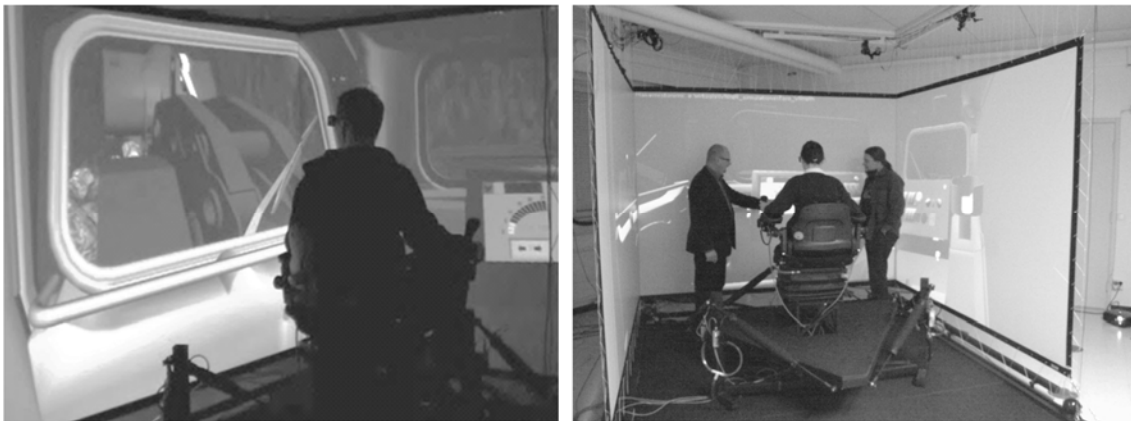
Figure 6. The view from the virtual cockpit of the mine loader machine and VE of the test 3
