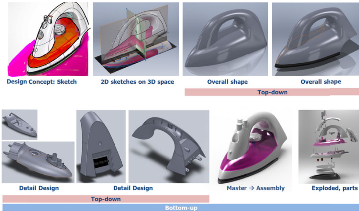
Figure 2. Top-down and bottom-up modelling approach
