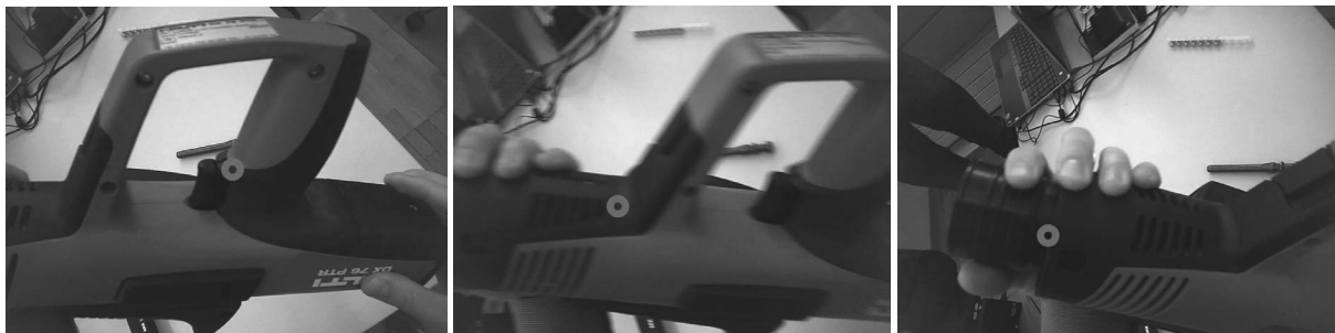
Figure 2. Eye tracking video of interaction with power tool; from left to right: sequence of gaze points (within 1,2 sec)
