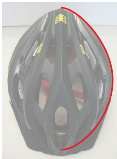
Figure 5. Parametric curve representing the footprint of a bicycle helmet with assumed symmetry
