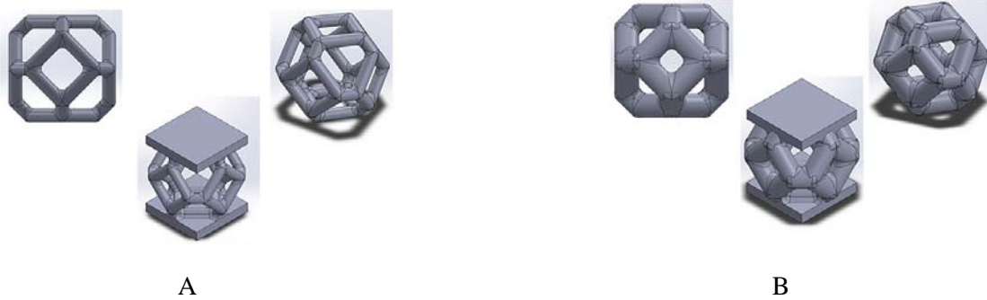
Figure 1. A: 1mm trabecular model B: 1.5mm trabecular model
