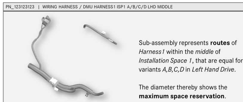
Figure 3. CAD sub-assembly of an automotive wiring harness
