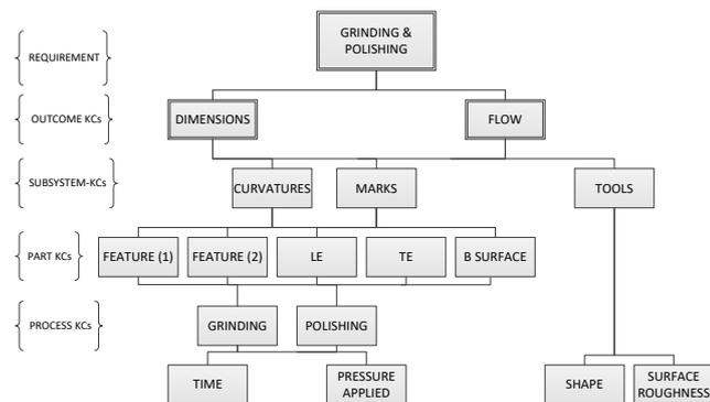
Figure 4. Key Characteristics (KCs) diagram (LE-leading edge, TE-trailing edge)
