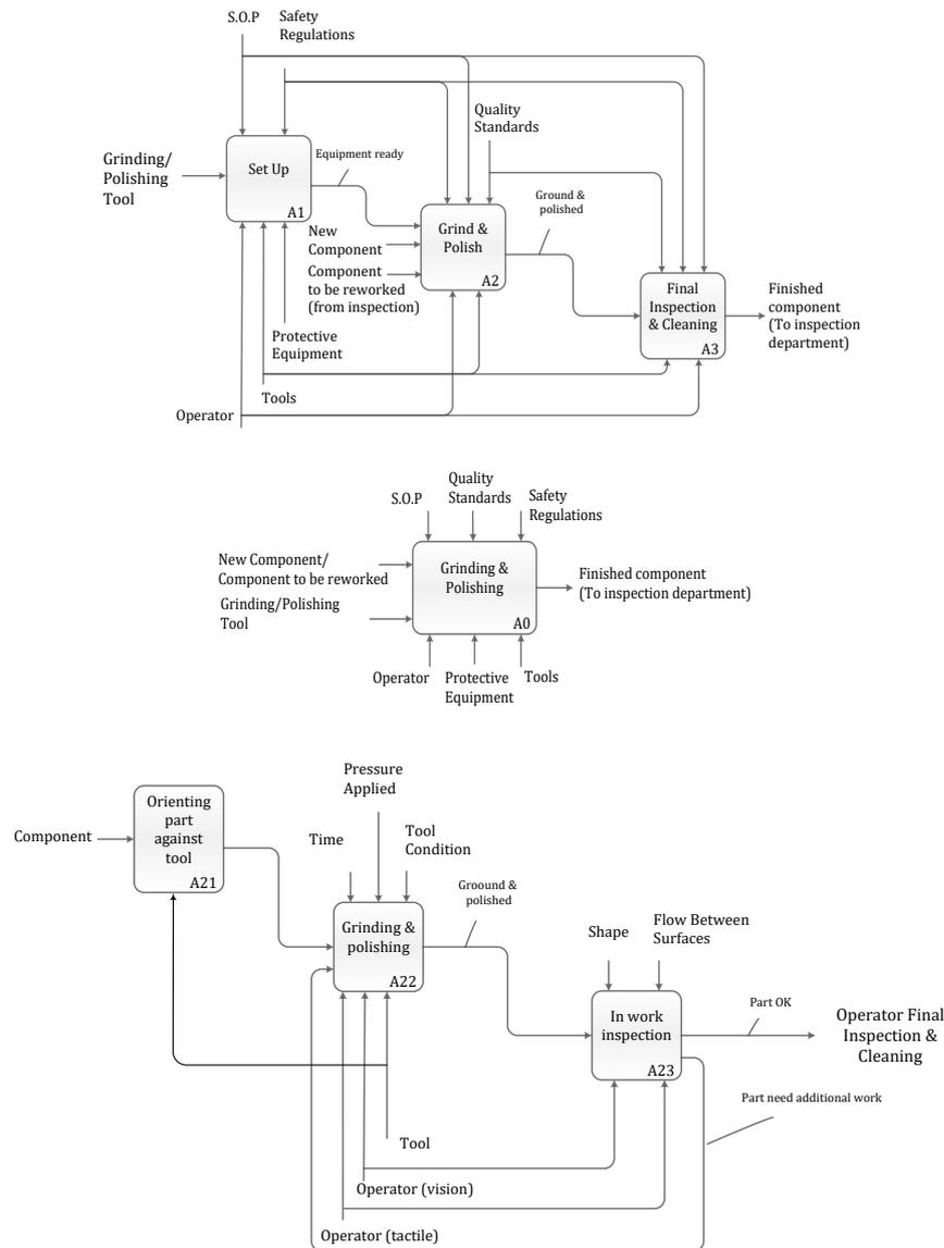
Figure 3. IDEF0 Diagram from process. A0 and A2 Level (only A2 is presented due to space constraint, all Controls apply to A21, A22 and A23; SOP and Quality Standards have been specialised further)
